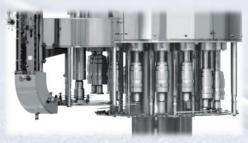
Rotary capping machine with magnetic clutch heads and Pick & Place device suitable to apply, on glass and PET bottles, **metal twist-off caps and plastic** pre-threaded screw caps with steam saturation inside bottles neck.
